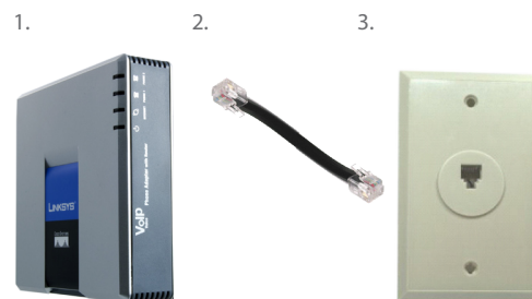
Figure 6: 1. Voice adapter, 2. RJ-11 Cable, 3. Standard RJ-11 Jack.
